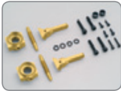
T44.6103-5 Aluminium front steering knuckles, L + R
